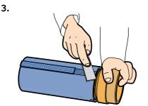
• Carefully file away the cable carrying strips until flush with the riser.
